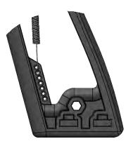
ATTACH SPRING TO SECOND HOLE FROM TOP OF TRIGGER FRAME
