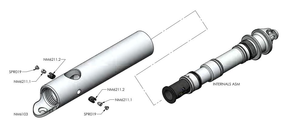
ENSURE SPR019 IS FULLY INSERTED INTO NM6211.2 AND REMAINS IN PLACE ON ALL FOUR TABS
