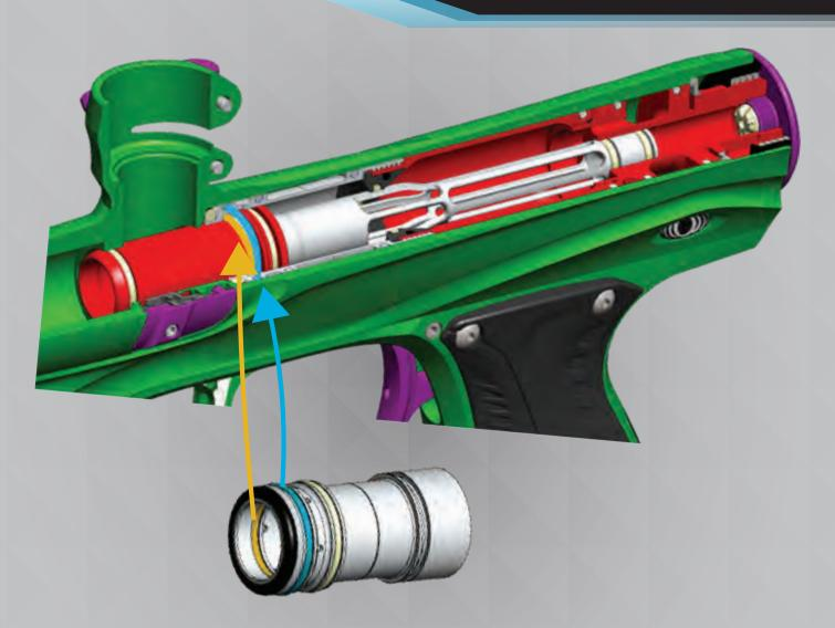
THIS DIAGRAM ILLUSTRATES THE O-RINGS RESPONSIBLE FOR AIR LEAKING AROUND THE OUTSIDE OF THE BOLD FACE.
